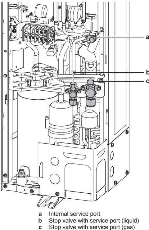
Typical workflow – Completely recharging refrigerant typically consists of the following stages:
